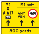
Lane restrictions at road works ahead
